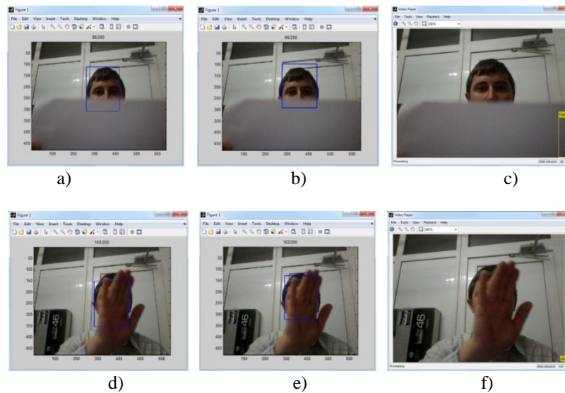
Fig. 5.23. Face tracking results in frames 86 and 163 from the second video sequence by using methods: CAMShift (a, d), MeanShift (b, e), Viola-Jones algorithm (c, f) [35]
