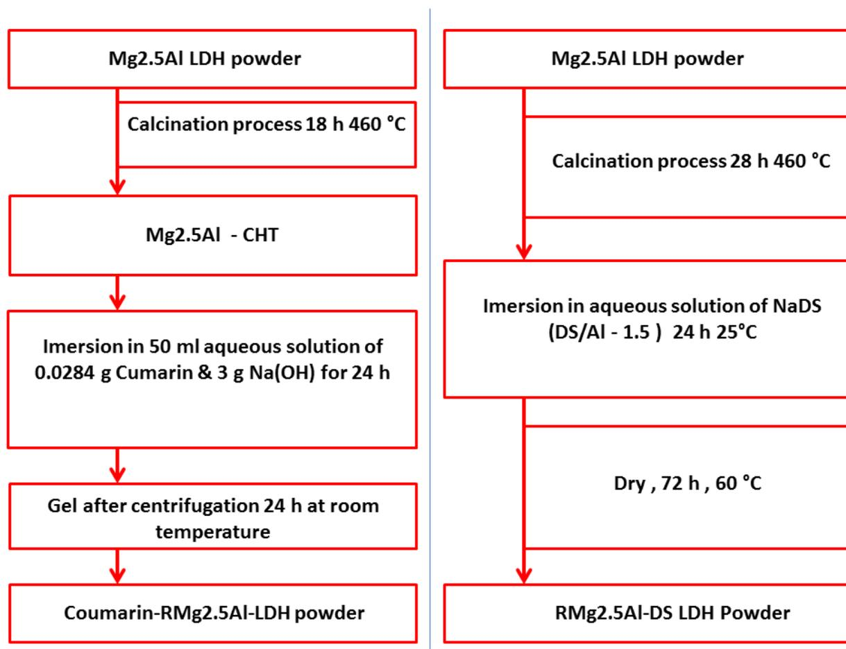
Figure 4.5 Schematic representation of the route followed for obtaining R-coumarin-Mg<sub>2.5</sub>Al-LDH and R -Mg<sub>2.5</sub>Al-LDH powder
