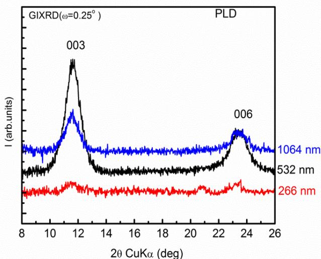
Figure 4.15 XRD patterns of the thin films deposited from the PMg 2.5 Al-LDH obtained using PLD at 266 nm, 532 nm and 1064 nm wavelengths
