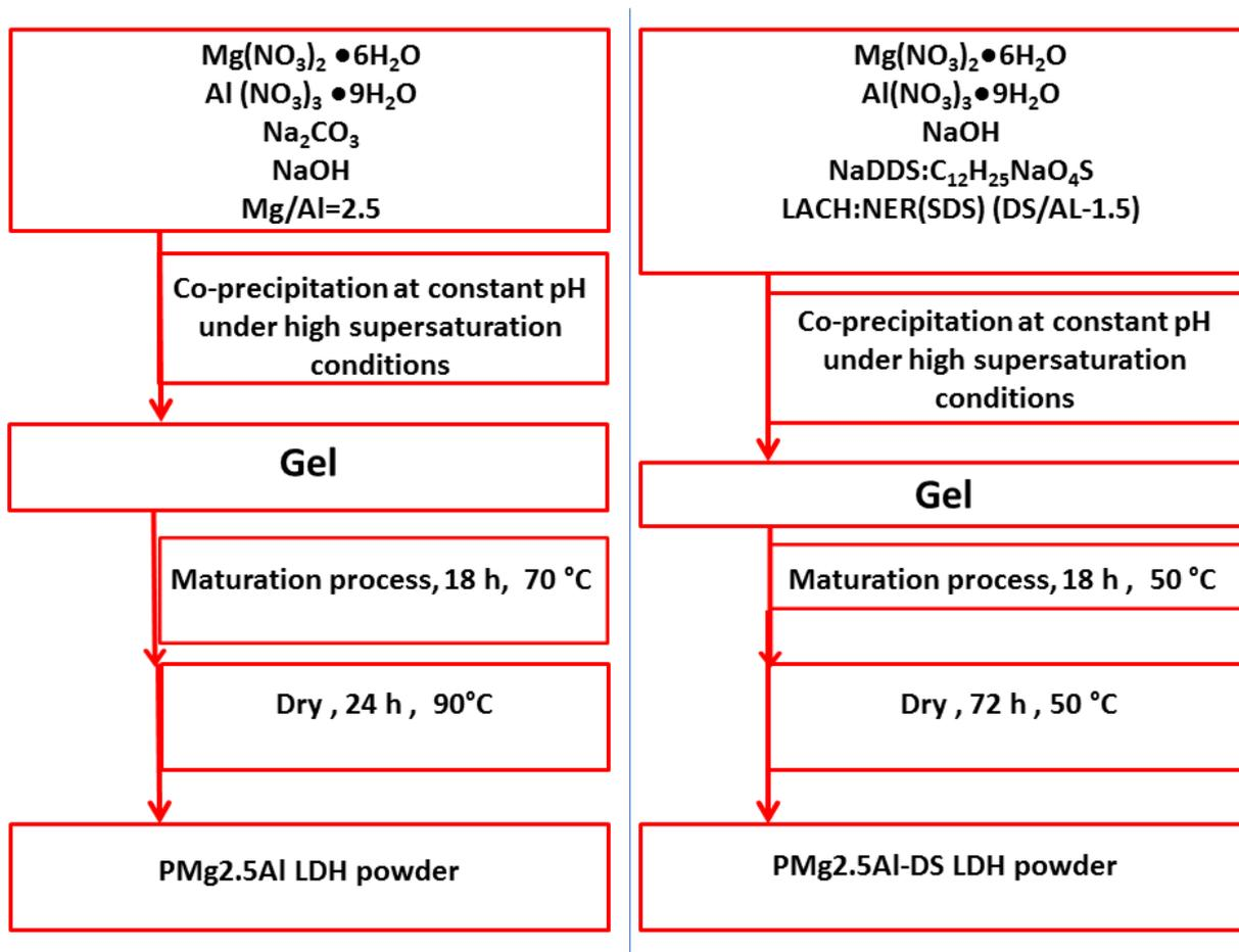
Figure 4.4 Schematic representation of the route followed for obtaining PMg<sub>2.5</sub>Al-LDH and PMg<sub>2.5</sub>Al-DS LDH powder
