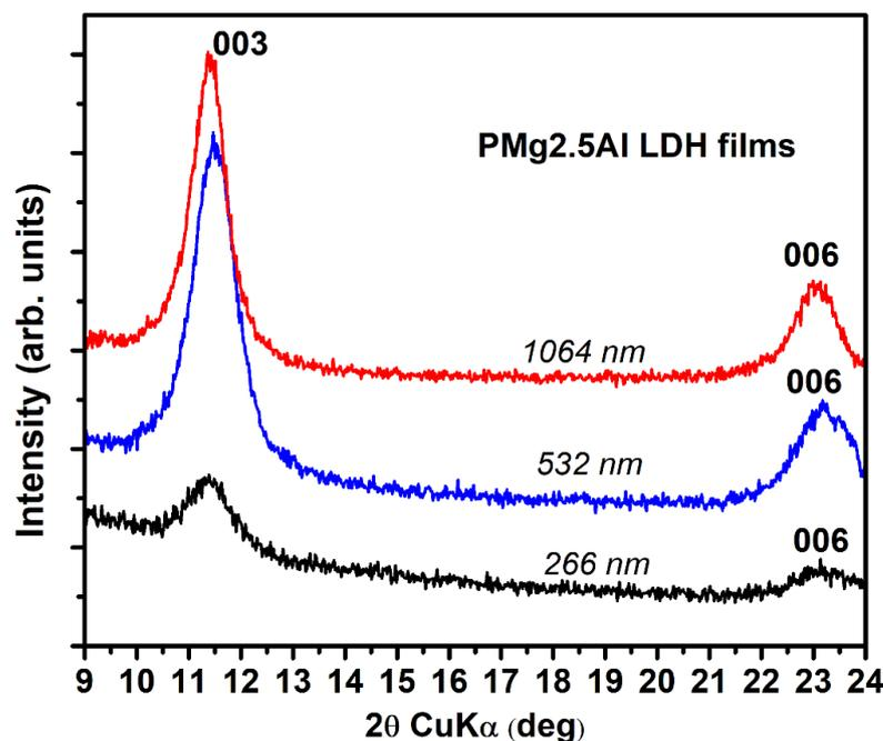
Figure 4.13 Representative XRD patterns of LDH thin films grown by PLD at 266, 532 and 1064 nm wavelengths
