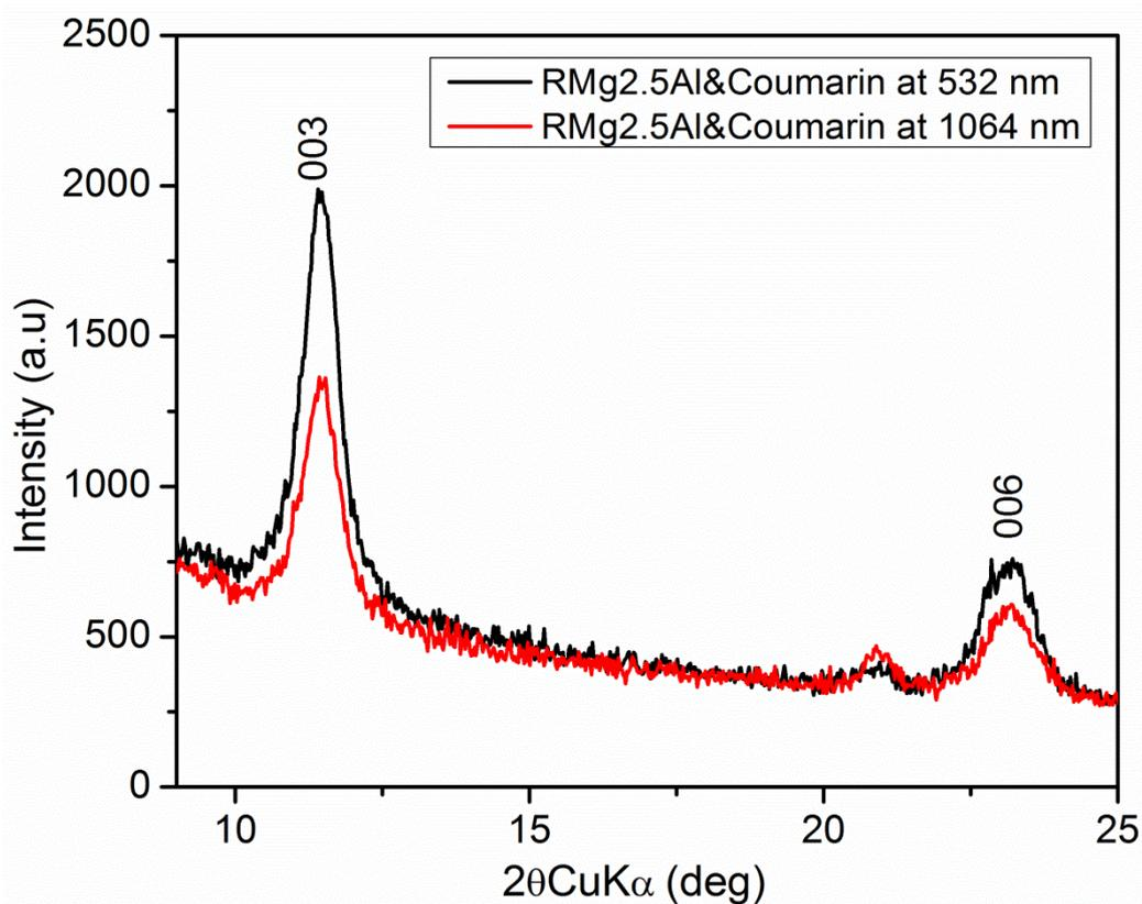
Figure 4.16 XRD patterns of the thin films deposited from the Coumarin-modified Mg<sub>2.5</sub>Al targets
