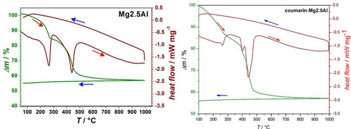
Figure 4.10 TGA and DSC diagrams of the Mg<sub>2.5</sub>Al-LDH and RMg<sub>2.5</sub>Al&coumarin LDH powders
