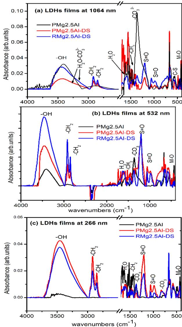
Figure 4.17 FTIR spectra of the PMg<sub>2.5</sub>Al-LDH, PMg<sub>2.5</sub>Al-LDH-DS și RMg<sub>2.5</sub>Al-LDH thin films deposited by PLD at different wavelengths: 1064 nm (Fig a), 532 nm (Fig b) and 266 nm (Fig c)
