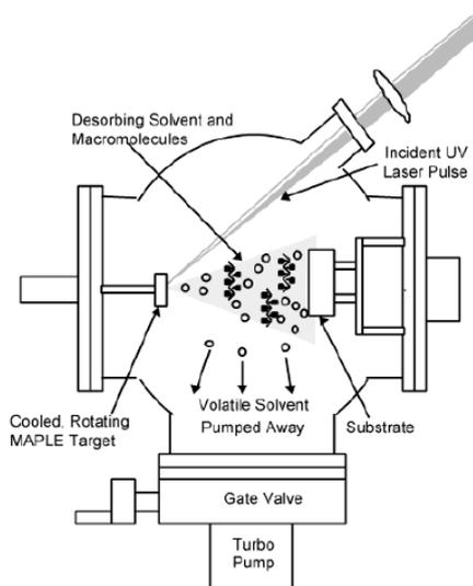
Figure 2.3 Schematic representation of the Matrix-Assisted Pulsed Laser Evaporation technique MAPLE [65]
