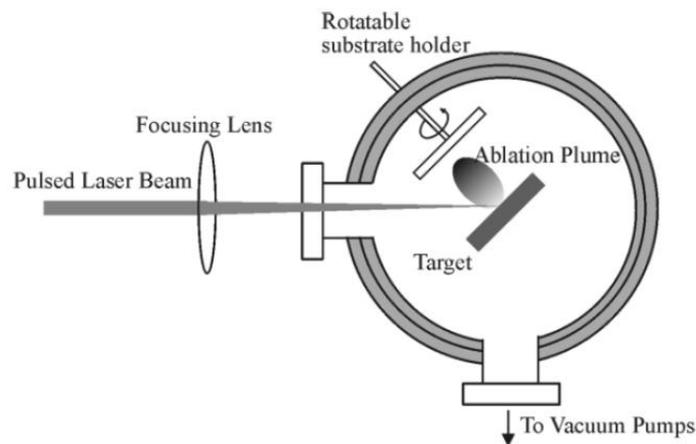
Figure 2.1 Schematic representation of the Pulsed Laser Deposition technique [48]
