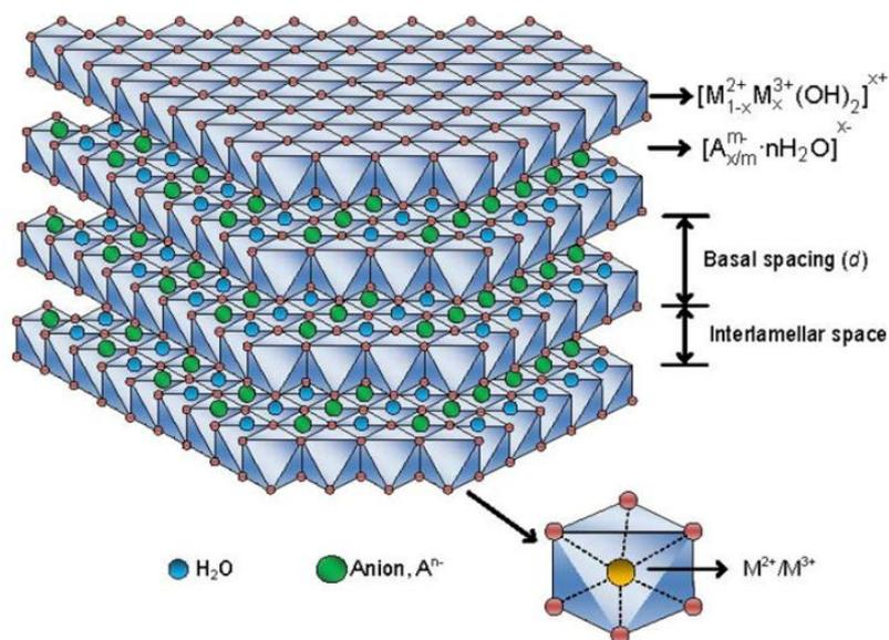
Figure 4.1 Schematic representation of the LDH structure
