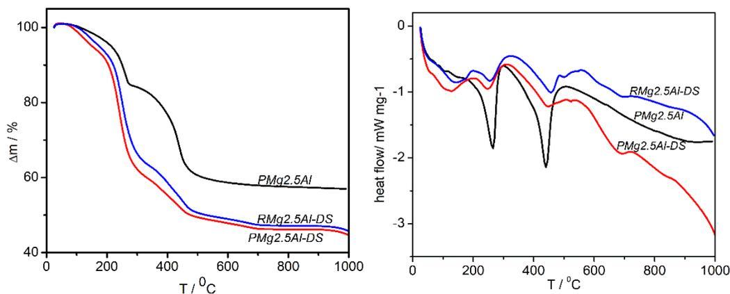
Figure 4.9 TGA and DSC diagrams of the as prepared DS modified LDHs and pristine LDH powders
