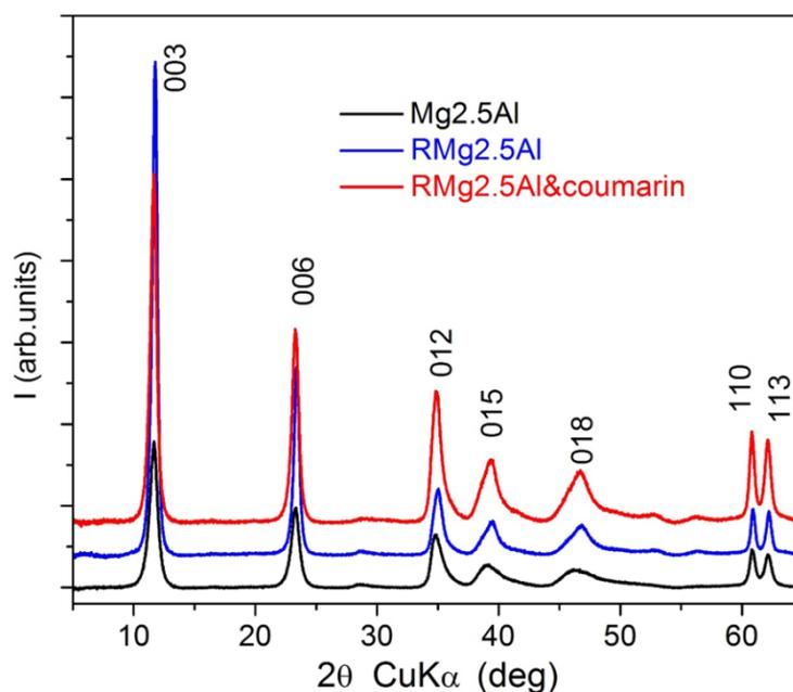
Figure 4.8 Representative XRD patterns for the powders Mg<sub>2.5</sub>Al-LDH, RMg<sub>2.5</sub>Al and RMg<sub>2.5</sub>Al&coumarin
