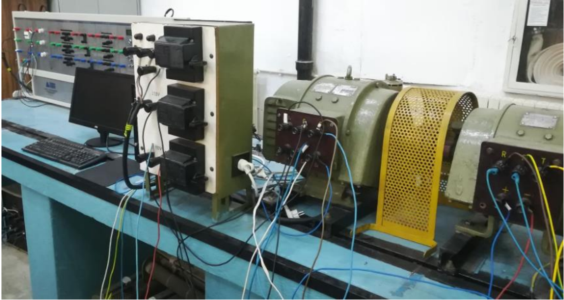
Fig. 6.1. The experimental stand for the active filtering and energy recovery systems for DC traction substations
