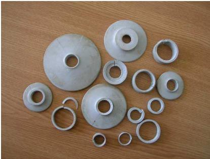
*Fig 1 – Silicone rubber recovered by milling and ripping*
