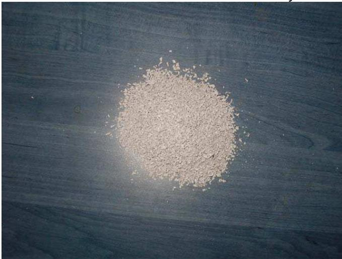
Fig. 5 – Silicone rubber powder
